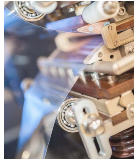
Roll-to-roll setup designed and built in-house at DIFFER, with the dielectric barrier discharge connected to the novel dual frequency power supply
