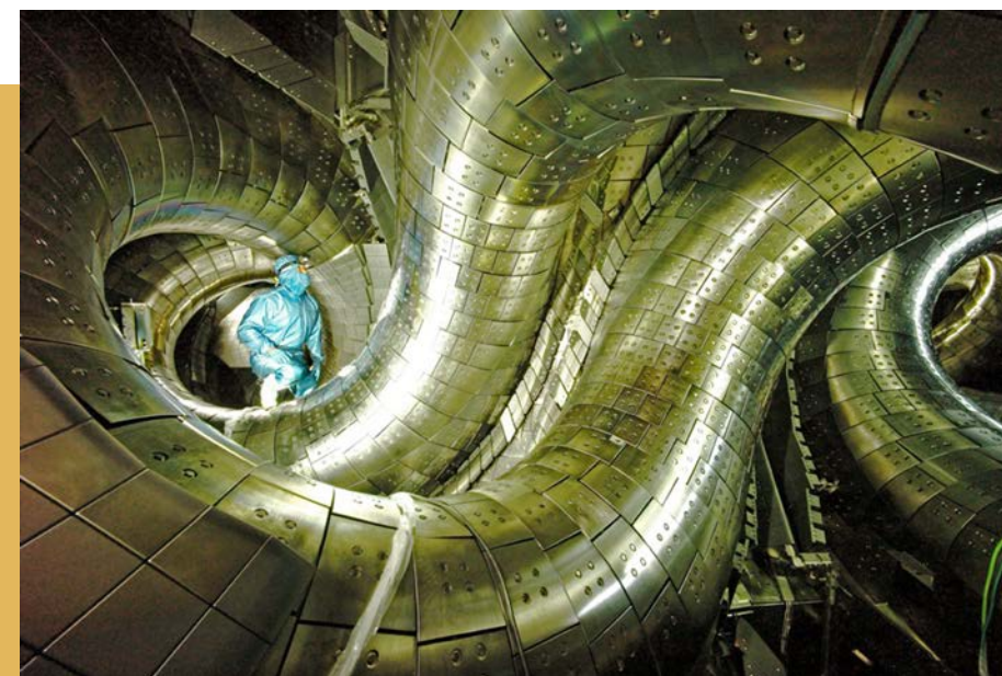
The Large Helical Device (LHD), a large superconducting stellarator (a type of fusion reactor) which can create long duration plasma discharges at temperatures of tens of millions degrees Photo: NIFS
