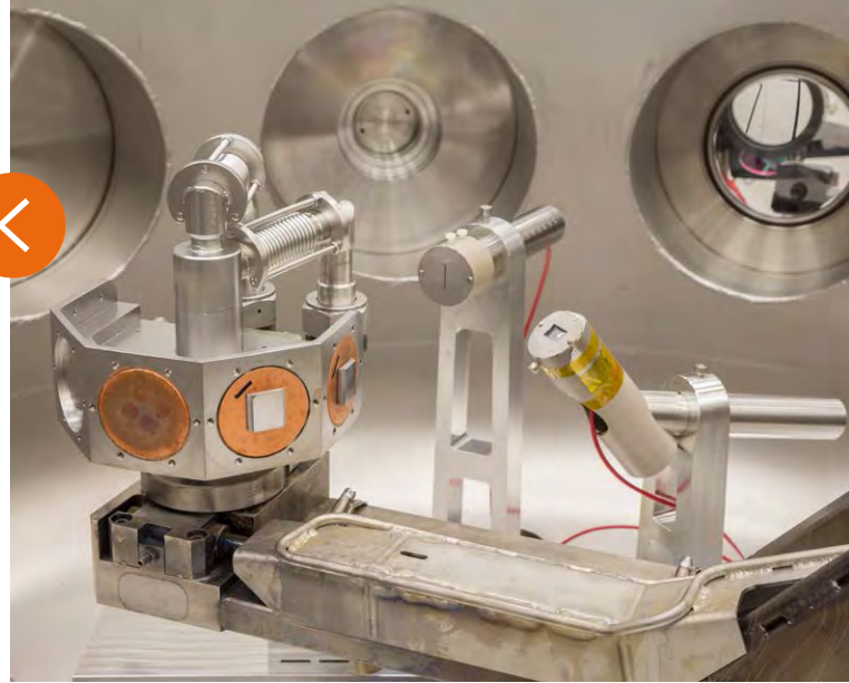
IBA detectors in the Magnum-PSI target exchange and analysis chamber, with target holder on the left.
