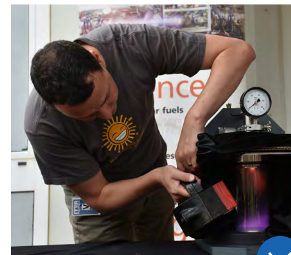
Showing that a magnetic field can shape a plasma at a distance (Photo: ITER)
