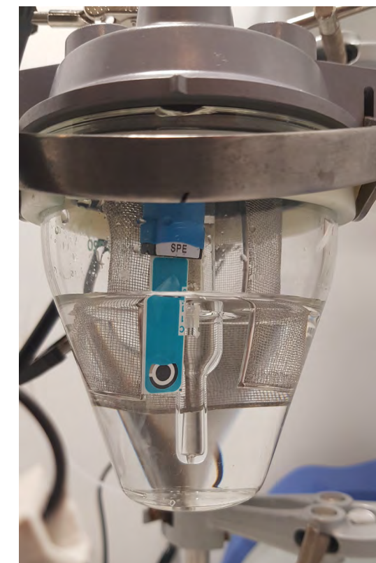
Fabrication and testing of a printed metal-oxide electrode
